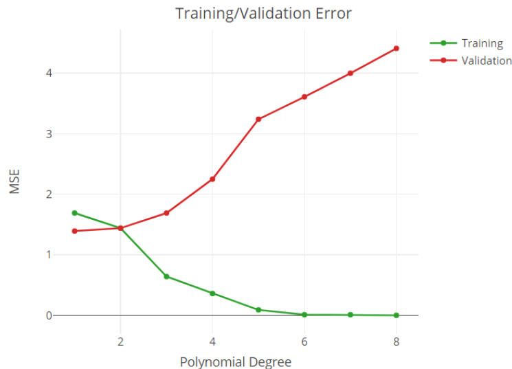
Figure 1.16: This graph contains the errors obtained from the data in Figure 1.15 (mean squared error), depending on the polynomial function employed. As we can see in Figure 1.15, the first-grade polynomial gives a larger error with respect to the eighth-grade polynomial in the training set , but a smaller one in the validation set .
