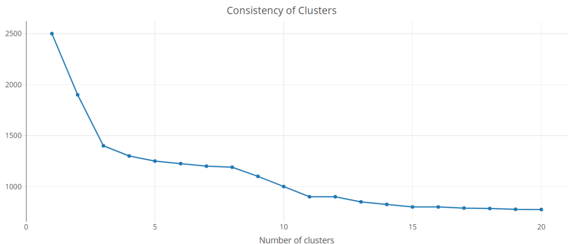
Figure 2.2: Graph analyses density, i.e. the closeness of the elements to each cluster, as the number of clusters K is increased.
